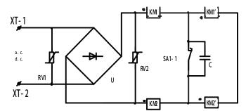
Fig: XT: wiring terminal; RV :varistor resistance;U :rectifier bridge ;SA :auxiliary switch ; C: capacitor; KM:coil start winding ; KM ': coil holding winding
