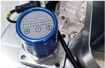
Liquid Level Sensor
