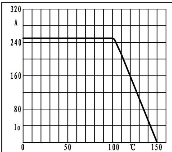
Fig5. Forward current derating curve
